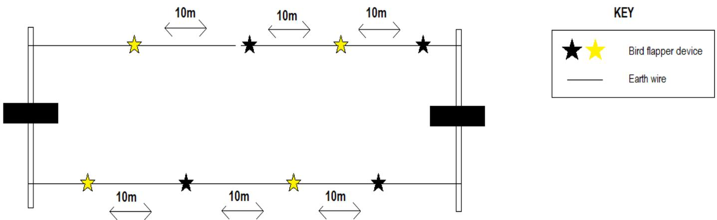
Technique and guideline for marking of the earth wire with bird flapper devices.
